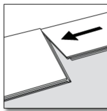
In the first row, place the second plank tight against the short end of the first plank.
