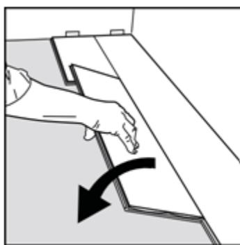
Place the plank at an angle against the plank in the previous row, press the edge forward against the previous row and fold down at the same time.
