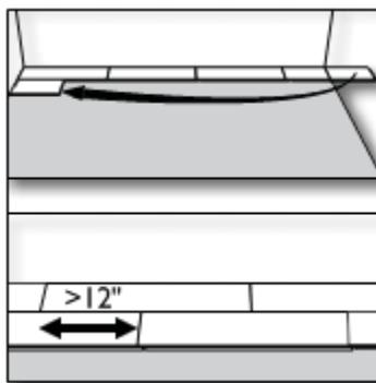
Place the plank face down on the work surface and cut to size with a power saw. If you are using a hand saw, use a fine-toothed blade, and cut the planks face up. The score/snap method (using a square or straightedge) requires the pad be cut from the back side using a utility blade (either before or after the score/snap).
