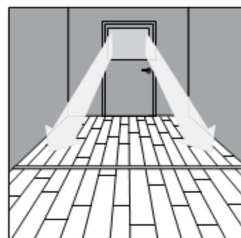
Try to run planks parallel to main light source.
