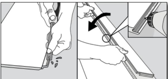
In areas such as a doorjamb or cabinet kick base where planks cannot be angled to lock into place, use a wood chisel to remove the locking ridge from the bottom of the plank groove.
