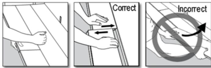
Separate the whole row by carefully lifting up and separating the whole row. Fold up and release the whole long side of the row, being very careful not to allow the planks to bend downward at the end seams! This could damage the locking mechanism of the plank!
