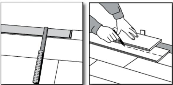
Measure and cut the last row to fit, remember to allow for a minimum of 1/4" expansion space from the wall. Use a full width scrap plank to mark your cutting on the last row.
